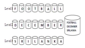
For example, if the 'A' bit of level 1 is lost then it is difficult to analyze from the single extra disk that the 'A' bit which is already there belongs to which level as two more 'A' bit is also used in level 3. Therefore, we are using extra disks in each level to analyze the data properly without being mismatching of data and the perfect data can be retrieved which is being lost.
